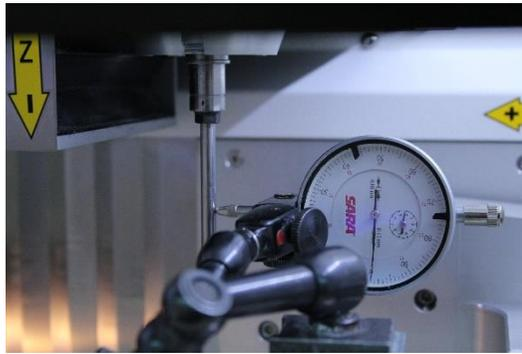
Attach the dial gauge with magnetic stand on the calibration blank.
