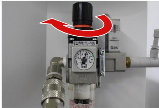
The inlet pressure of the machine must be set to 6,5 bar by turning the regulator.
