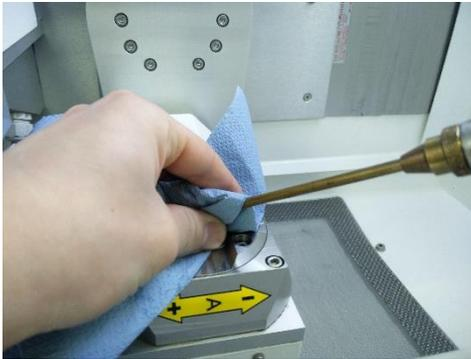
The creeping oil must act for at least ten minutes. The creeping oil is blown with compressed air gun into a cleaning cloth.
