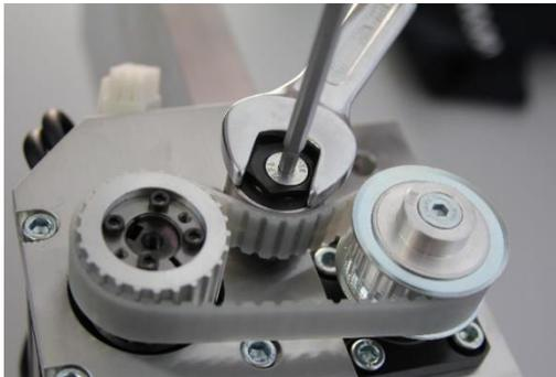
Install the timing belt, tensioner and M6 countersunk screw. The M6 countersunk screw must be tightened hand-tight. The toothed belt is then pretensioned by turning the tensioning roller with the open-end wrench. The timing belt should then move about 6-8 mm. Finally, the M6 countersunk screw of the tensioner pulley is tightened.
