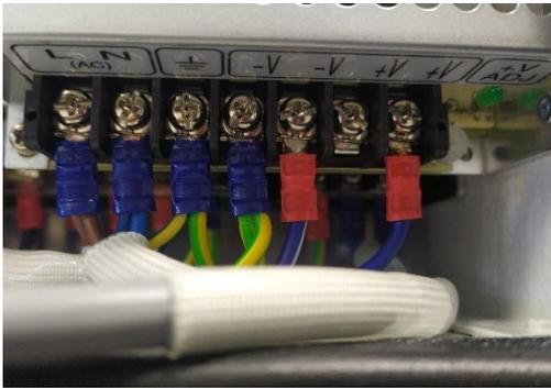
Connect the cable lugs of the single wires.
