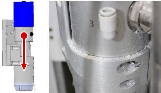
Insert the new spindle in the spindle clamp. The spindle must flush straight to the clamping block.
