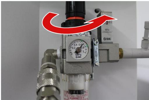
Set the main pressure of the machine to 7 bar by turning the regulator.
