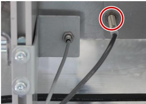
After loosening the M8 counter nut the switching distance can be adjusted.
