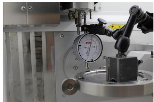
Attach dial gauge and magnetic stand to calibration blank and cover of milling spindle.
