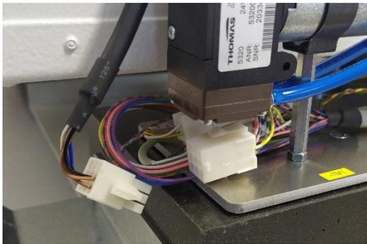
Disconnect the nine-pin AMP connector of the safety interlock cable.
