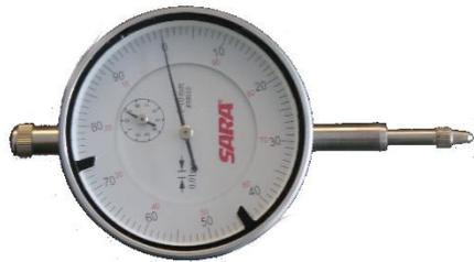
Check the deviation from the zero position. If the pointer deflection is outside the tolerance of 0.02 mm, the mechanics must be controlled.
