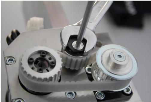
Install the timing belt, tensioner and M6 countersunk screw. The M6 countersunk screw must be tightened hand-tight. The toothed belt is then pretensioned by turning the tensioning roller with the open-end wrench. The timing belt should then move about 6-8 mm. Finally, the screw of the tensioner is tightened.
