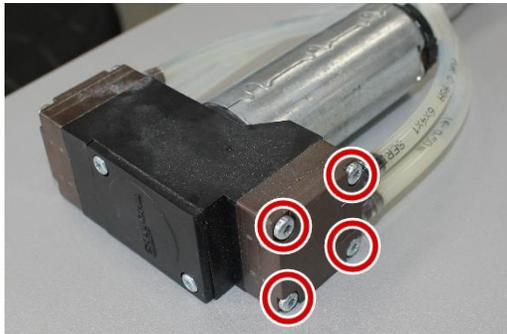
Mount the four M4 Torx screws (T10) and the cover on the right side of the diaphragm pump.
