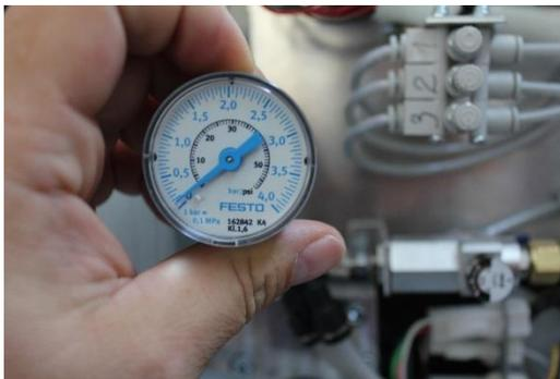
Check the pressure on the manometer.
