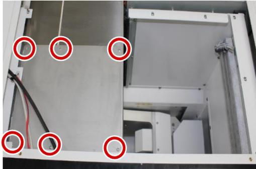
Remove the six Phillips screws and the service flap of milling spindle.
