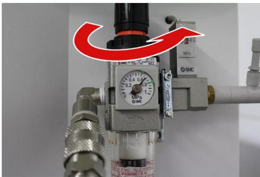
Set the main pressure of the machine to 6,5 bar by turning the regulator.
