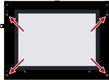
Remove the four mounting bolts. Following this, the remaining four M3 cylinder head screws are bolted to the position of the mounting bolts.
