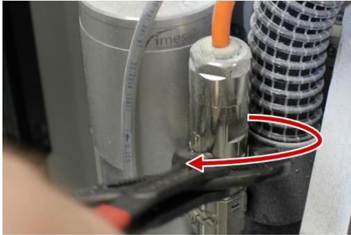
Attach the connection cable of the spindle.
