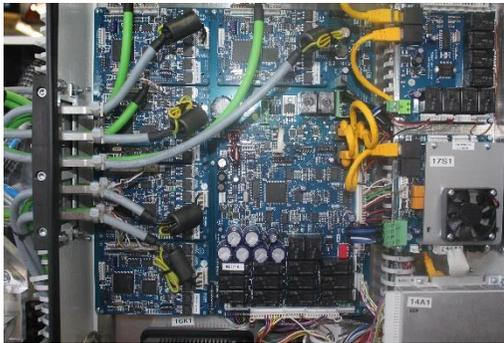
Connect all cable connections and jumper of the 5 axis CNC BUS Controller.
