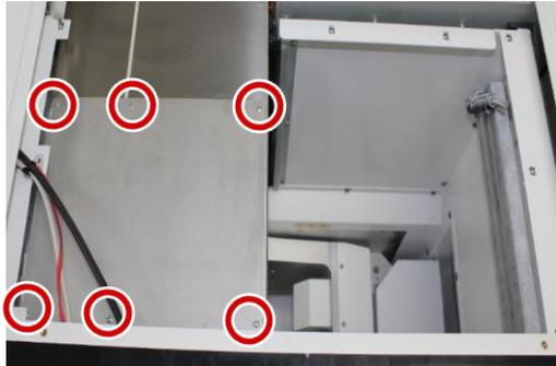
Mount the six Phillips screws and the service flap of milling spindle.
