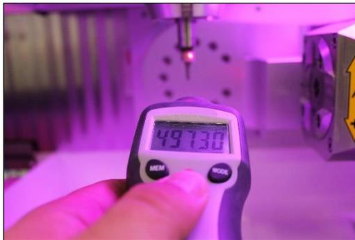
Switch on the rev counter. After that the laser aimed at the calibration pin and note the current speed.
