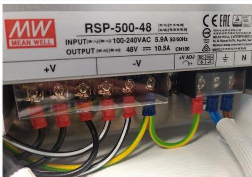
Photograph the pin assignment of the power supply unit.
