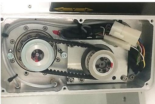
Connect the connector of the A-Motor and fasten with cable ties.
