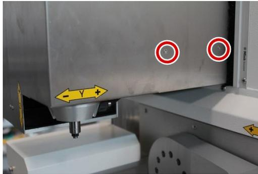
Remove the two M3 countersunk screws.
