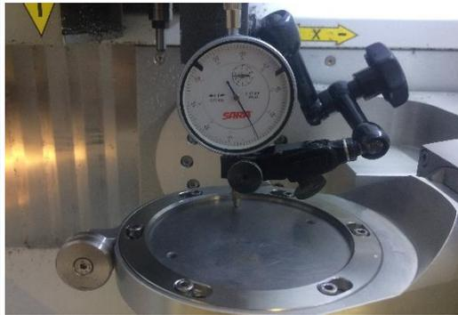
Attach dial gauge and magnetic stand to plate for magnetic stand. The measuring tip of the dial gauge should be in the rear and center of the calibration blank.
