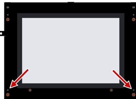
The door must be opened until it stops. Afterwards the two lower M3 cylinder head screws are fixed.
