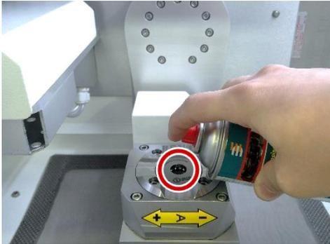
Spray creeping oil into the zero-clamping system. Never use alcohol or aggressive cleaners!
