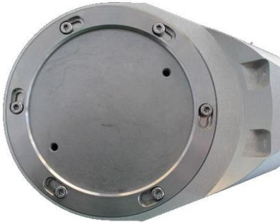
Clamp the calibration blank in the machine.
