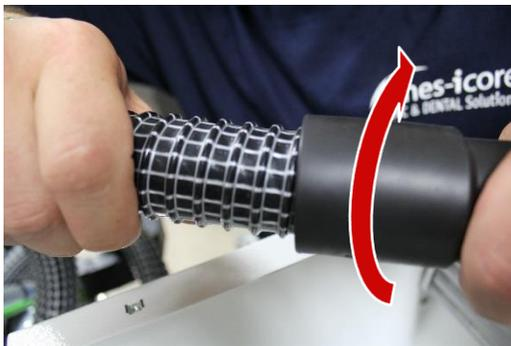
Screw adapter piece onto new suction hose.
