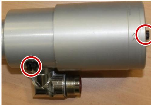
Mount the two compressed air connections (old spindle) to the new spindle. The two blind plugs must be mounted on the old spindle.
