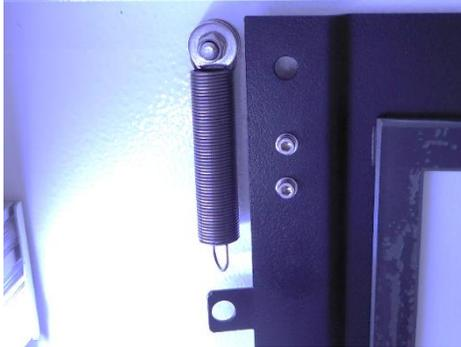
Unhook the spring from the protective door. The following steps are executed in the interior.
