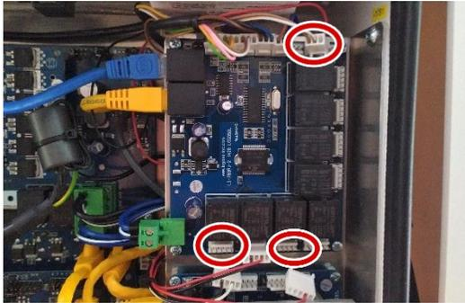
Disconnect the three connectors from the IO module.
