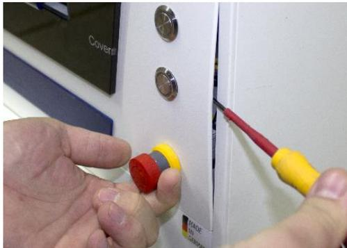
By slightly pulling out the EMERGENCY STOP switch, the operating unit can be levered out.
