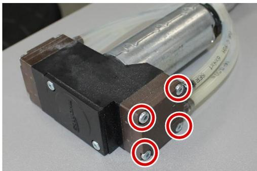
Remove the four M4 Torx screws (T10) on the right side of the diaphragm pump.
