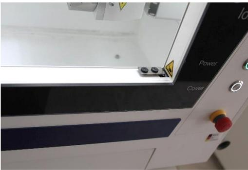
Bridge the safety door on the milling room with the clamp door lock.
