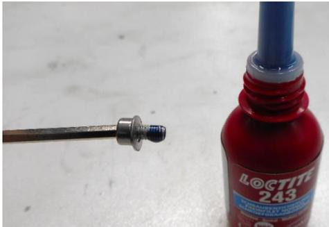
Preparation of four M3 cylinder head screw with a washer (small) and thread locker, as shown in the picture.
