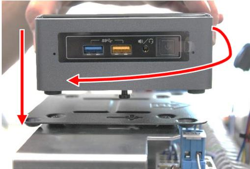
Carefully place the computer on the holes in the holder and turn it clockwise.
