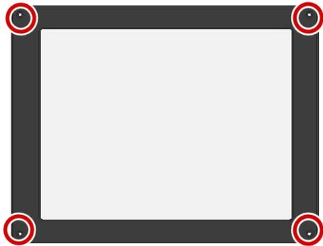
Remove the four M3 countersunk screws.
