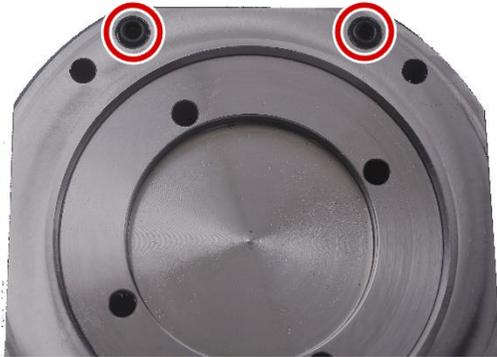
Insert sealing rings into the marked holes of the new zero-point clamping system.
