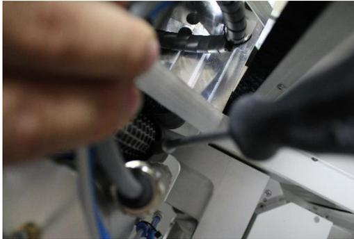
The adapter piece of the new suction hose must be pressed into the extraction nozzle with the socket wrench.
