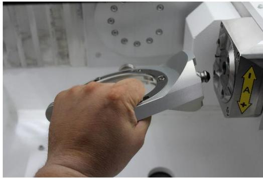
Remove the blank holder out of the zero-point clamping system.
