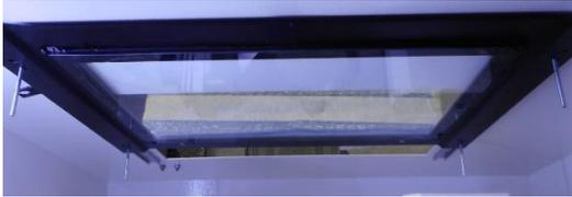
Insert the new safety gate onto the bolts (the bolts must be in the lower holes of the safety door).
