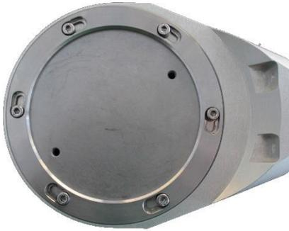
Clamp the calibration blank in the machine.
