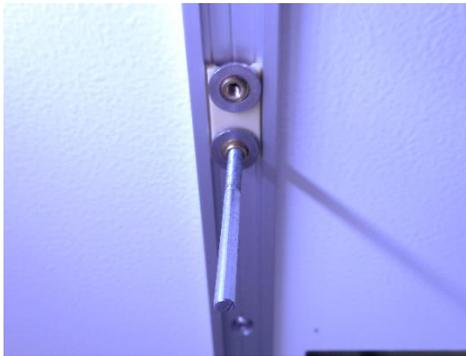
Attach the four new sliding bushes with washer (large) to the lower thread with one mounting bolt.
