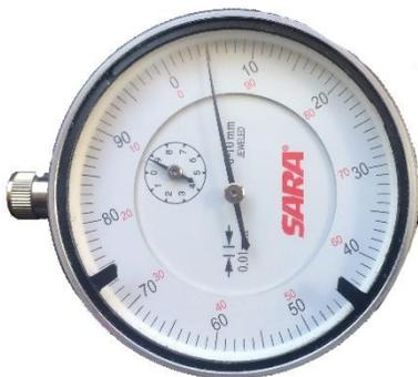
Check the deviation. If the deviation is higher than 15  $\mu\text{m}$ , steps 4. - 13. must be repeated.
