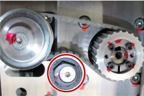
Untighten the pretention of the tensioner pulley.
