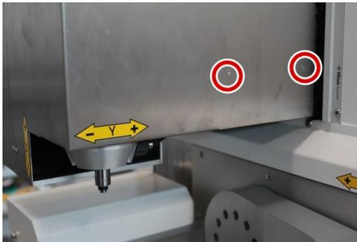
Mount the two M3 countersunk screws.
