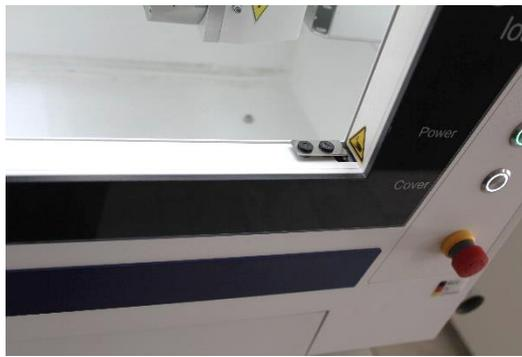
Bridge the safety door on the milling room with the clamp door lock.
