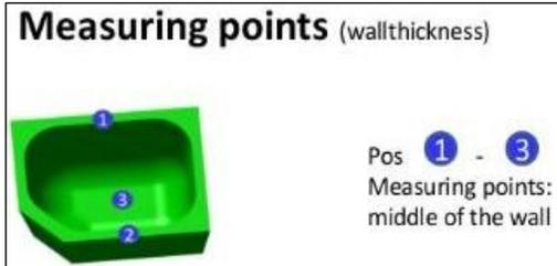
Measure the wall thicknesses 1, 2 and 3 with an accuracy of 0.01mm.
