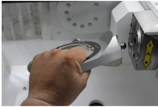
Insert blank holder in the zero-clamping system.
