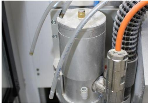
Remove the hoses. Press the retaining ring on the compressed air connection while the hose is being pulled out.
