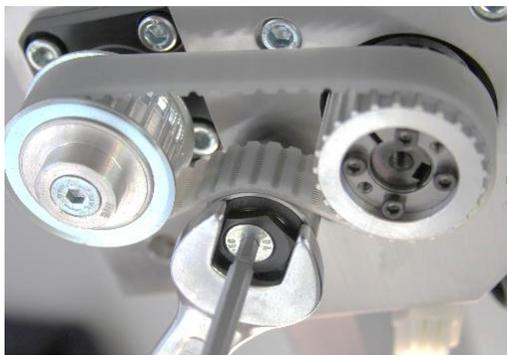
Mount and tension the M6 countersunk screw and tensioner. After that the timing belt must be allowed to move 6 - 8 mm.
