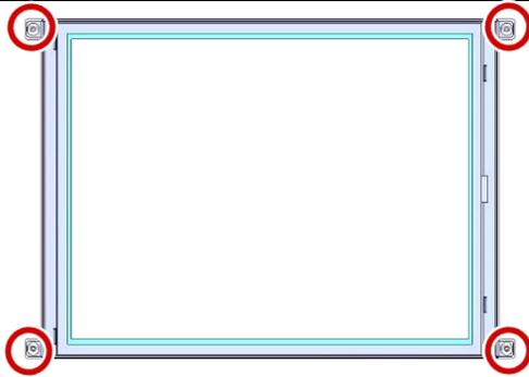
Remove the four M5 pan head screws.
