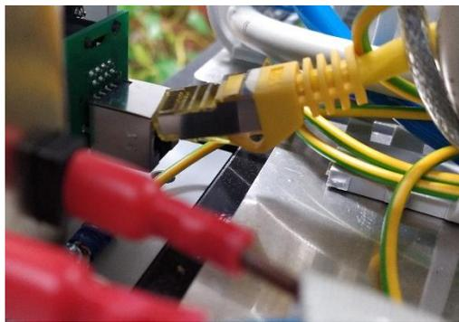
Disconnect the network cable from the network connection.
