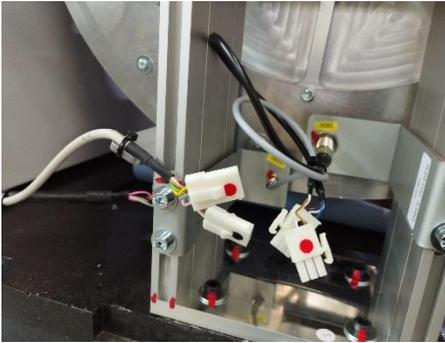
Mark and disconnect the plugs of the two loader wheel sensors. If there are no plugs, disconnect the two cables in the switchgear.
